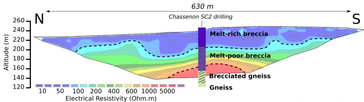
**Figure 1:** electrical resistivity cross section over the Chassenon butte and the 120 m deep SC2 drilling, and associated geological interpretations.
