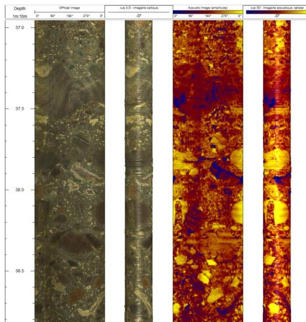
Figure 1. Examples of unrolled and rolled high resolution optical and acoustical images acquired in hole SC2. The images are oriented with respect to magnetic North. Depth is given in meters below ground level.
